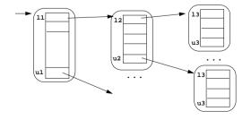
Each single array can be allocated separately, dynamically; scattered in memory In **Java arrays** are implemented this way.
