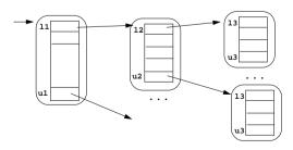
Each single array can be allocated separately, dynamically; scattered in memory In **Java arrays** are implemented this way.
