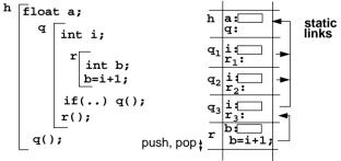
The **static link** points to the activation record where the called function is defined, e. g. r<sub>3</sub> in q<sub>3</sub>
