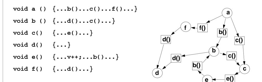
Calls of the same function in different contexts are distinguished by different nodes, e.g. the call of c in a and in b.
